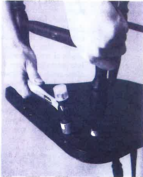
64-6. Use a mallet to dismantle furniture pieces without damage.
