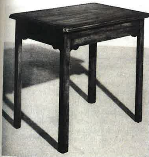
49-1. This table is a good example of leg-and-rail construction.
