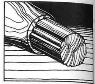
48-8(a). The compression spindle makes a permanent joint for turned parts.
