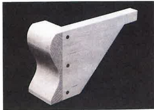
48-27. This is a section of the back foot showing how the flat bracket is attached.
