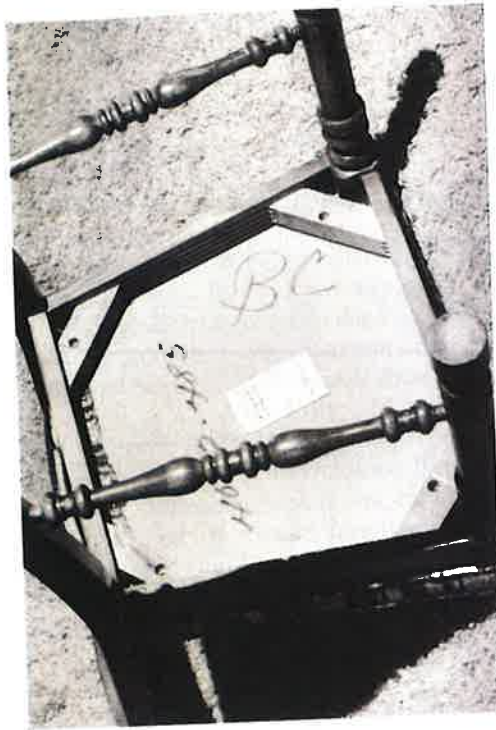
49-9. Butt joints with dowels are used on this chair. Note that the corners are not square. The corner blocks are grooved to increase the holding power of the glue.
