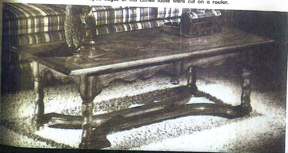
33-3. The shaped edges of this coffee table were cut on a router.
