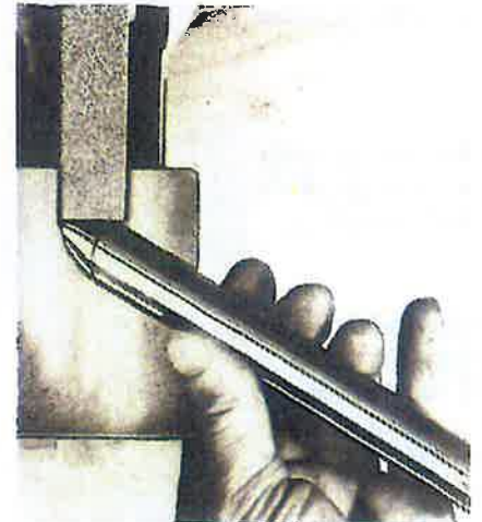
24-21. Grinding a gouge on the face of a slipstone. In this method, the tool must be rolled to keep the same angle of bevel all around the tool.
