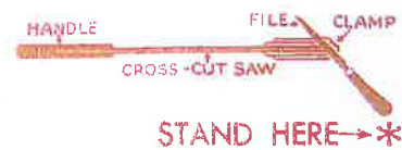
24-32. Second position for filing a crosscut saw.
