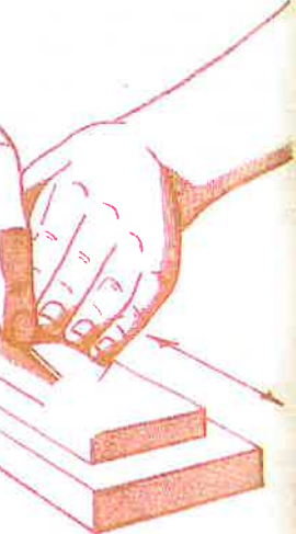
Plane iron blade by moving it back and forth in a straight line.
