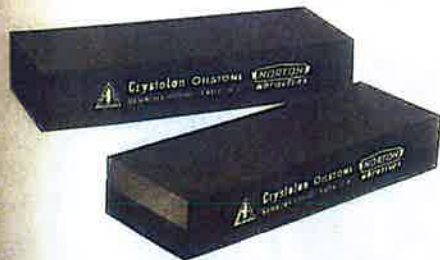
24-4. Artificial abrasive bench stones. Their advantage is that a combination stone can be made, one side coarse and the other fine.
