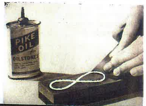
24-9. Another method of honing the edge is to move the tool in a figure-eight pattern.
