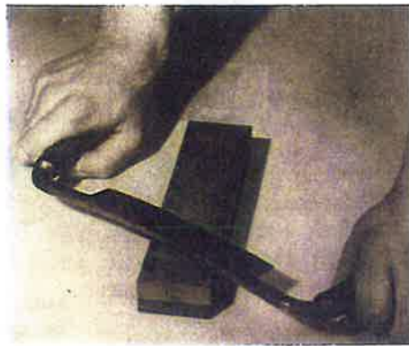
24-14. Honing the cutting edge of a draw knife.
